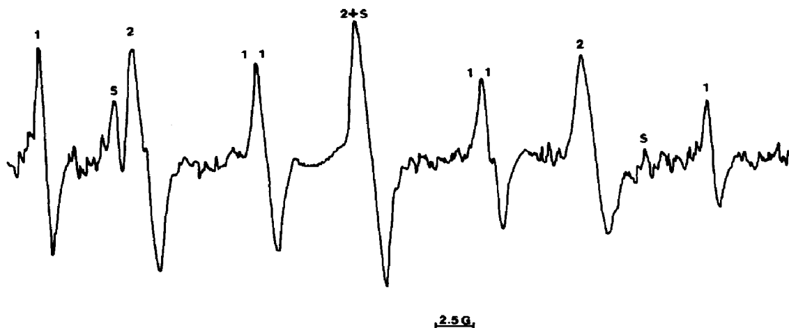
Fig. 1. The ESR spectrum observed during irradiation of nitrogen-saturated aqueous solution of DAA ( 10^{-3} M) in the presence of NtB ( 1 \text{ mg ml}^{-1} ).
